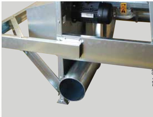
Screenings are conveyed through pipes up to 50' (15m) away
