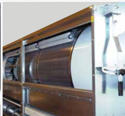
The cleaning brush role is mounted on a spring-loaded arm-securing efficient even load on the cleaning brush
