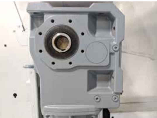
Gear with parallel shafts makes it easy to turn drum by hand, makes screen change easier
