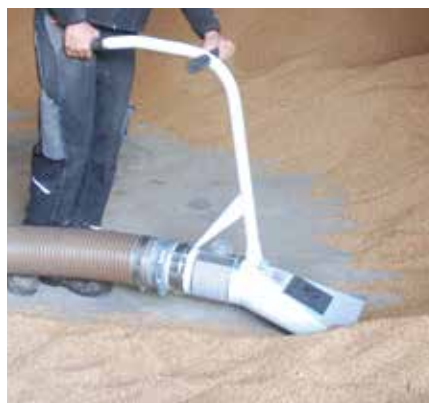
Suction head for cleaning purposes: Easily picks up the last remnants of grain on the floor.
