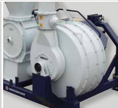
Automatic air control is standard on tractor-powered blowers.
