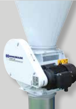
CAE 20 rotary valve mounted below the cyclone in a pure suction installation.
