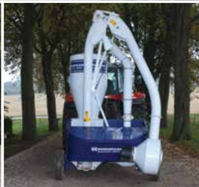
Loading equipment hydraulically folded to transport position.
