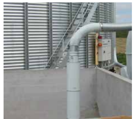
Long suction head: Suitable for conveying from grain pits.
