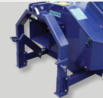
Three-point attachment to tractor lift.
