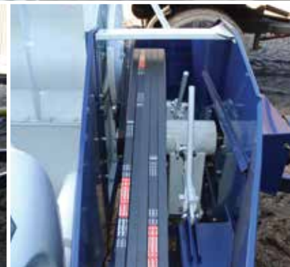
The belts can be tightened without using tools, although tools are required to gain access to the belts.
